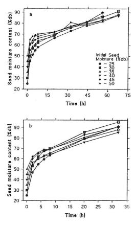
Fig. 2. Water uptake curves for wheat seed of different initial moisture content germinated at two temperatures:  $12 {}^{0}C(a)$  and  $30 {}^{0}C(b)$ . Open symbols indicate 90 % seeds germinated.
