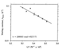
Fig. 4. Mean wetting constant  $(k_{mean})$  tor the group of water uptake curves at each hydration temperature.
